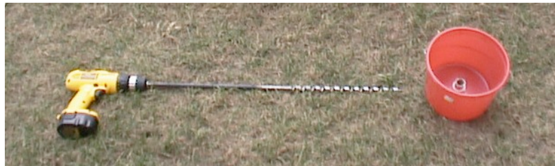
Figure 1. The sweatless soil sampler developed by the Soil, Water and Forage Analytical Laboratory at Oklahoma State University.
